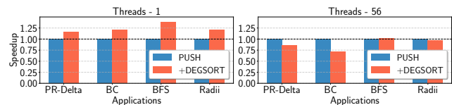
Figure 3: Performance improvements from Degree Sorting: Reordering improves performance of a single-threaded execution but fails to provide speedups for parallel executions.
